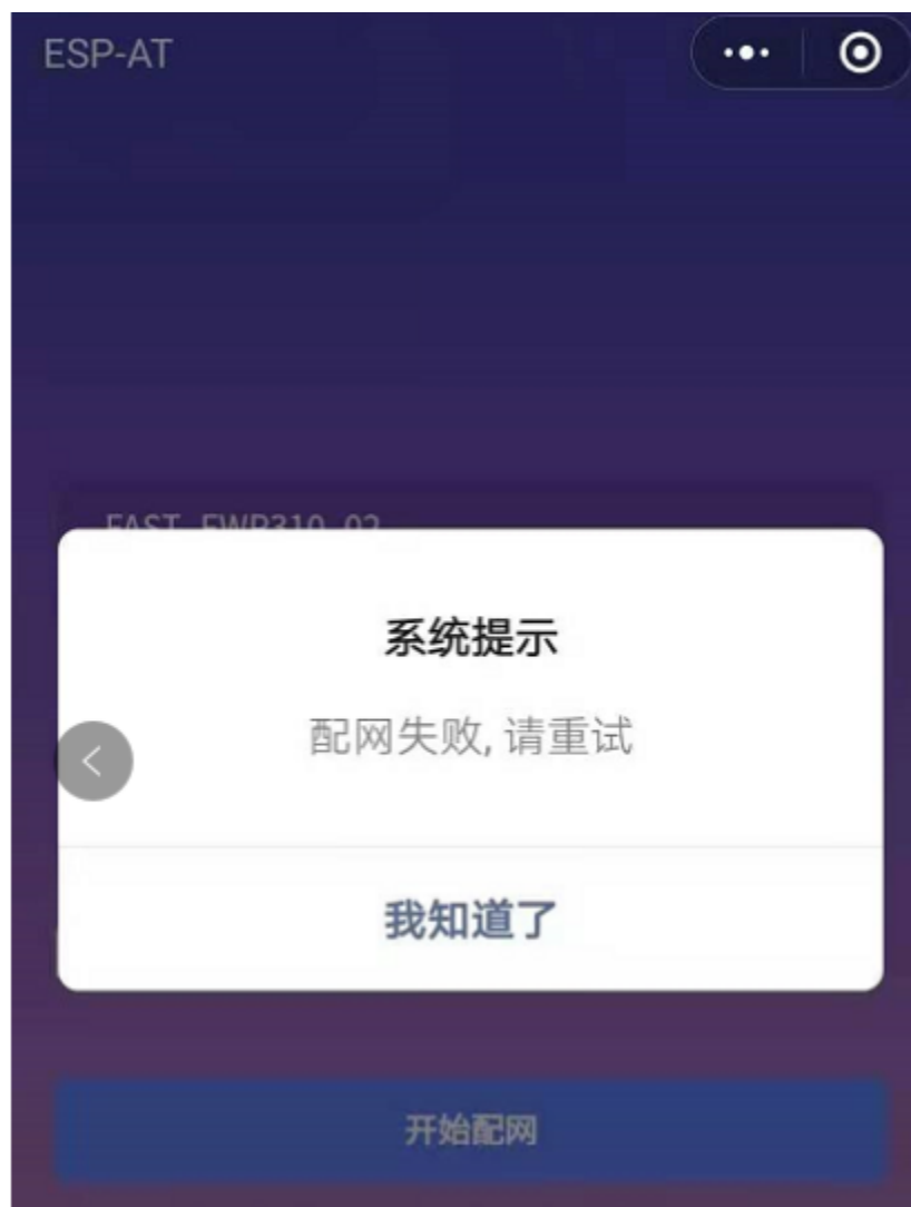
Fig. 16: The applet Wi-Fi provisioning is failed
